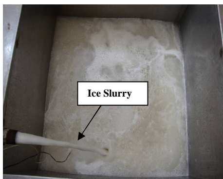
Fig. 8: Photographs of Ice Slurry of -11.9^{\circ}\text{C} formation in SSISG using MEG
